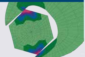
Conventional open end wrench: edge pressure causes surface damage
