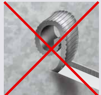
Notching without chip breaking
