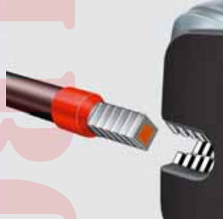
Square crimping for optimum contact zones
