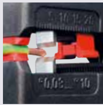
Precise stripping prevents damage to the conductor
