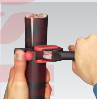
Turning the tool for circular cut
