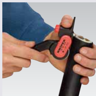
Setting the tool for longitudinal cut
